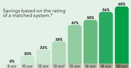
\* Based on Energy Star's Savings Calculator for a 3-ton 20 SEER/10HSPF heat pump and programmable thermostat versus the industry standard 13 SEER/7.7 HSPF 3-ton heat pump and standard thermostat in St. Louis, MO.
