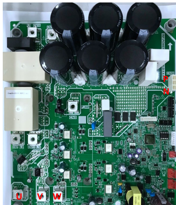
Figure 6-2.1: Inverter module terminals
