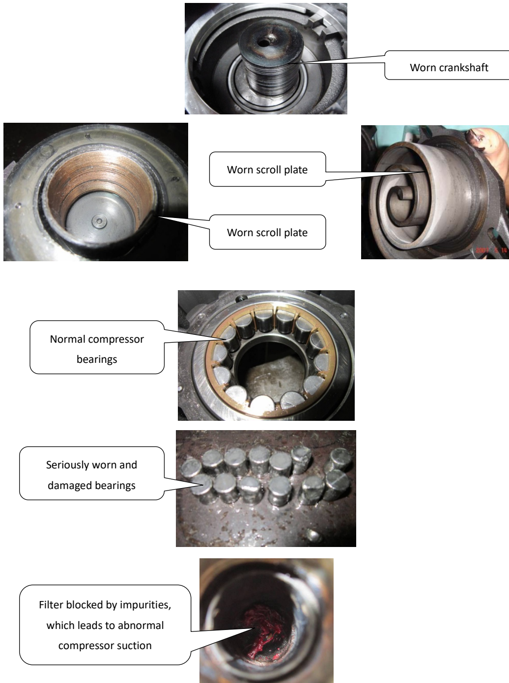
Figure 6-2.11: Effects of spoiled compressor oil
