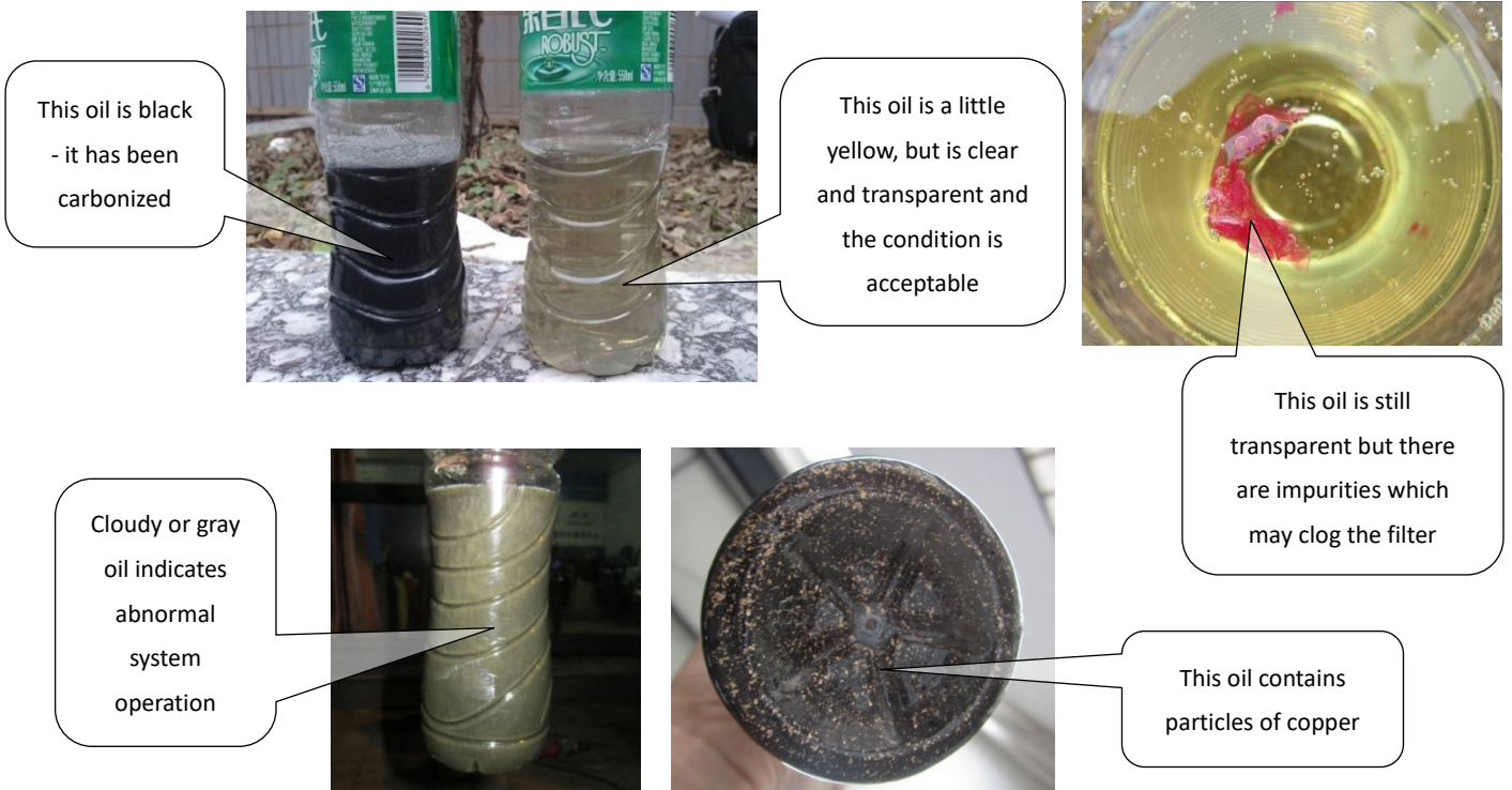
Figure 6-2.10: Inspecting compressor oil
