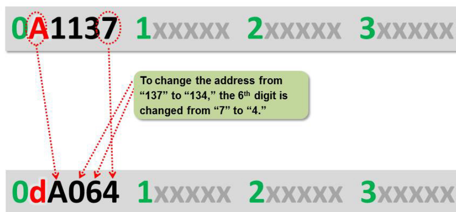
Figure 10. Example of using the specific digit changing mode to change a unit address
