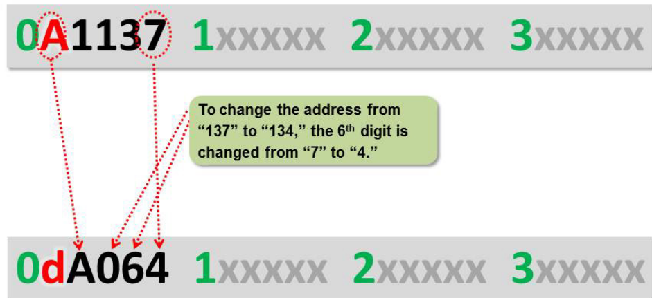
Figure 10. Example of using the specific digit changing mode to change a unit address
