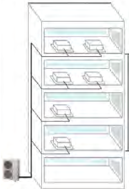
Figure 24. Maximum vertical change between outdoor unit and highest indoor unit
