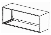
General Electric Plastic Wall Sleeve; remove bottom seal from plastic sleeve.
