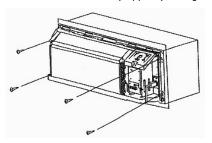
6. Re-install front panel by first, hooking tabs over top rail of unit and then pushing in on the bottom of the front panel until it snaps into place.
