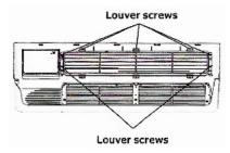
$2. \quad \text{Remove louver screws that hold the louver insert in place on the back side of the front panel}.$
