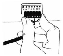
4. Connect wires from the thermostat to terminals on unit terminal connector.
