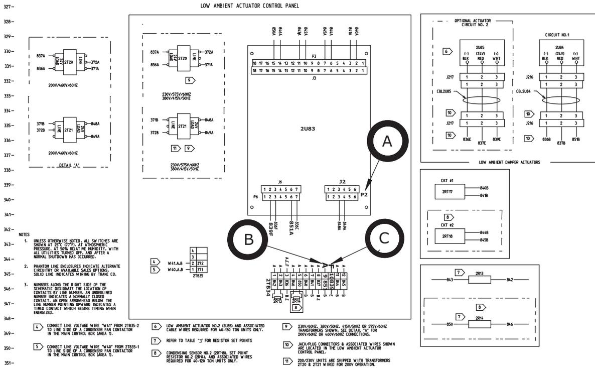
**Figure 24. Instructions — CAUJ condenser control circuit modification:
