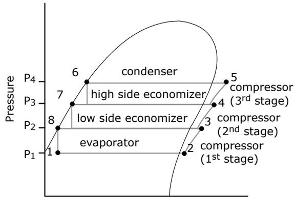
**Figure 35. Refrigerant flow, 3-stage**
