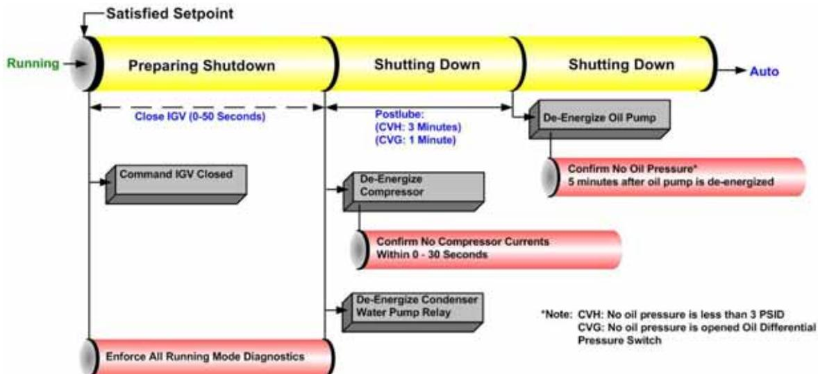
If the STOP key is pressed on the operator interface, the chiller will follow the same stop sequence as above except the chilled water pump relay will also open and stop the chilled water pump after the chilled water pump delay timer has timed out after compressor shut down (see Figure 47).
