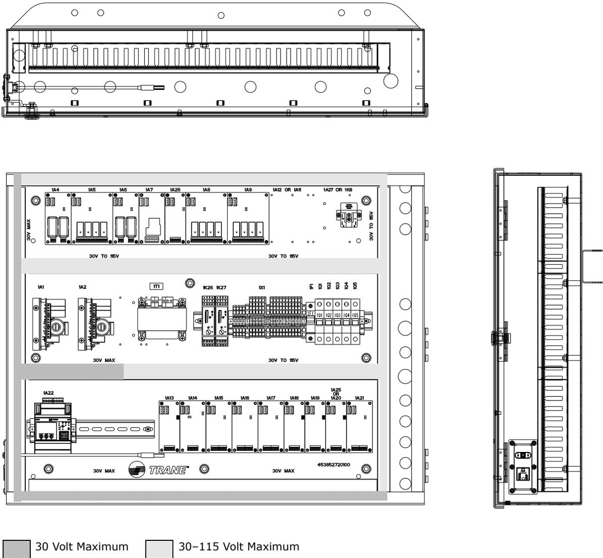
Figure 27. Standard control panel: Tracer AdaptiView main unit assembly right hand panel (showing low voltage and higher voltage areas for proper routing of field wiring)
