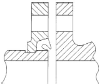
3. Align and bring two pipe ends together and slide gasket into position centered between the grooves on each pipe. No portion of the gasket should extend into the groove on either pipe.
