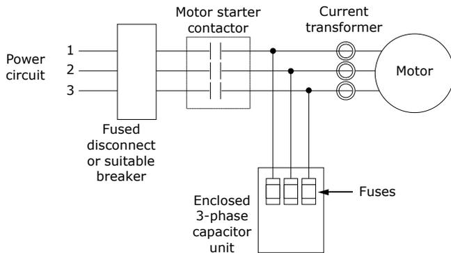
**Option 1—PFCCs installed downstream of starter contactor, upstream of current transformers.**
