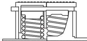
6. Check the clearance on each isolator. If this dimension is less than 1/4 in. (6.35 mm) on any isolator, use a wrench to turn the adjusting bolt one complete revolution upward.
