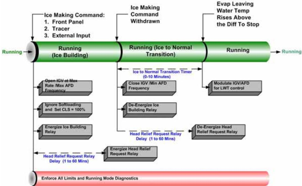
Figure 49. Sequence of operation: ice making: stopped to ice to ice building complete
