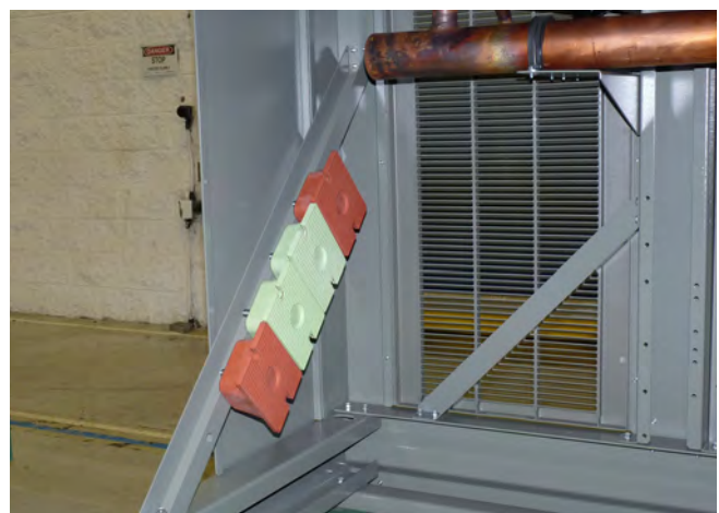
Figure 4. Elastomeric isolators attached for shipping
