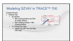
So let's talk about how to model this system in TRACE 700. By default TRACE sets the min stop at 30% of the design supply airflow. This value can be overridden to meet requirements for your system.
