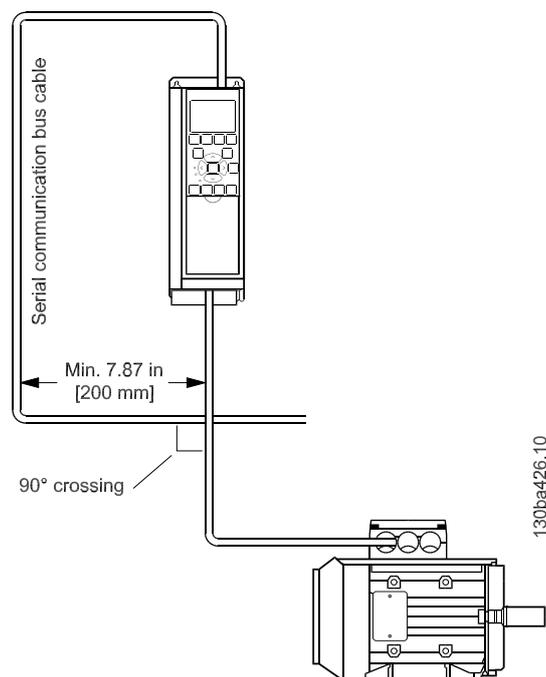
It is highly recommended to use suitably shielded cable for any LonWorks installation!
