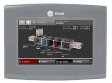
The Tracer<sup>™</sup> TD7 Display features a touch-sensitive color screen that provides for ease of viewing and editing of Tracer UC600 data. Building operators can easily monitor space temperature and relative humidity, change setpoints, and enter point overrides with time-limits with a just a few touches of the screen.
