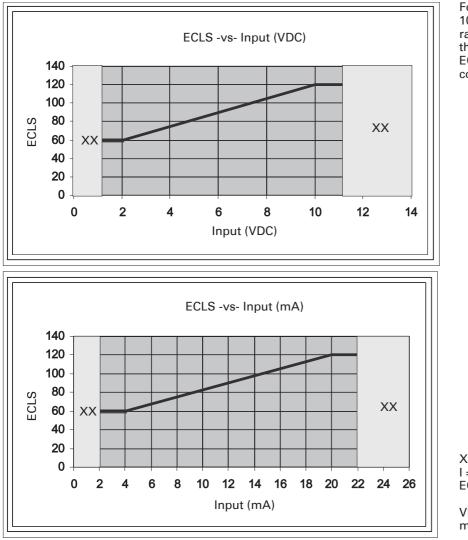
For input signals beyond the 2-10VDC or 4-20mA range, the end of range value is used. For example, if the customer inputs 21 mA, the ECLS limits it self to the corresponding 20 mA ECLS.
