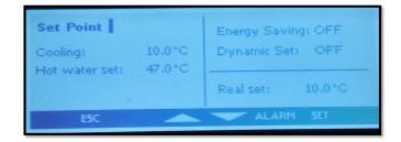
With this function you can change the set point in order to ensure, to changing external conditions, increased comfort or higher efficiency of the unit.
