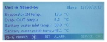
In case the unit is controlled by remote or during shutdown by time slot, the main screen will be:
