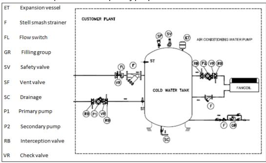
IMPORTANT: The flow switch in the customer plant is obligatory in order to keep the warranty. Install the flow switch with a minimum of 5 times the pipe diameter of straight horizontal run on each side. Do not install close to elbows, orifices or other valves.
