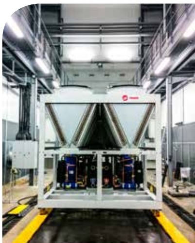
CMAC HE unit on our Charmes (F) laboratory test loop
