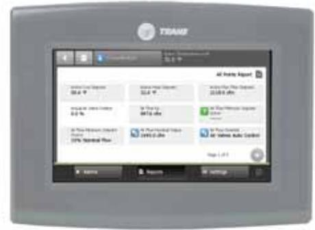
The Tracer™ TD7 Display features a touch-sensitive color screen that provides for ease of viewing and editing of Tracer UC600 data. Building operators can easily monitor space temperature and relative humidity, change setpoints, and enter point overrides with time-limits with a just a few touches of the screen.
