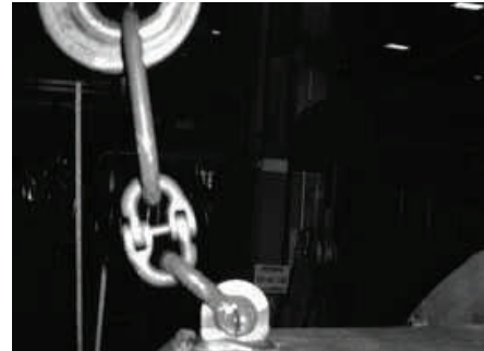
Figure 15. Lifting clevis on the suction elbow lifting tab (three-piece elbow style)
