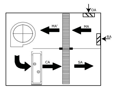
The Trane CDQ wheel uses a Type III desiccant (activated alumina) chosen specifically for this application. The ability of the desiccant to adsorb water vapor is very high when the relative humidity of the air is high (see Figure 6).
