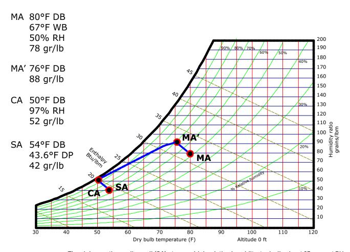
The air leaves the cooling coil (CA) at a very high relative humidity, typically about 97 percent RH. The CDQ desiccant wheel adsorbs water vapor from this air stream, removing 10 grains of water per pound mass of air in this example. This adsorption process results in the addition of some sensible heat, raising the dry-bulb temperature of the supply air (SA) by 4°F in this example. The mixed air entering the regeneration side of the wheel is at a lower relative humidity (50 percent).
