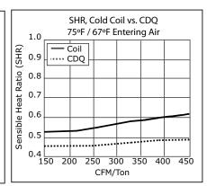
This reduction in unit SHR is not accomplished by adding heat. It is a result of increasing the latent capacity of the coil with the CDQ wheel. This increase in latent capacity is achieved without increasing the total capacity. Figure 13 is the same data represented in terms of latent capacity improvement. The latent capacity improvement at the examples conditions range from 15 to 550 percent.
