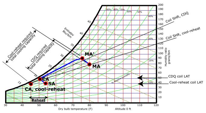
The cooling coil SHR, sensible heat ratio (the ratio of sensible cooling to total cooling), is also lowered with a CDQ system without using reheat. This helps the unit better match building loads, especially during part load conditions and reduces the need of reheat. The temperature gain from the wheel is minimal, typically 3°F to 9°F, thus the system can cool and dehumidify.
