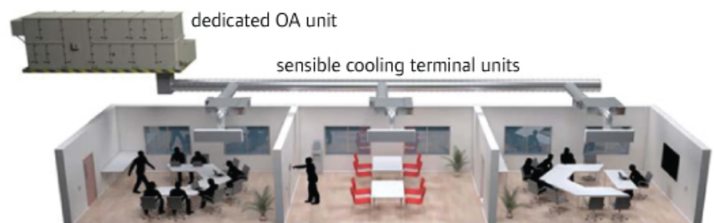
Figure 1. DOAS with chilled-water, sensible-cooling terminal units
