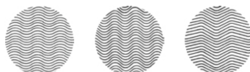
Figure 2. Typical geometries for coil fins
